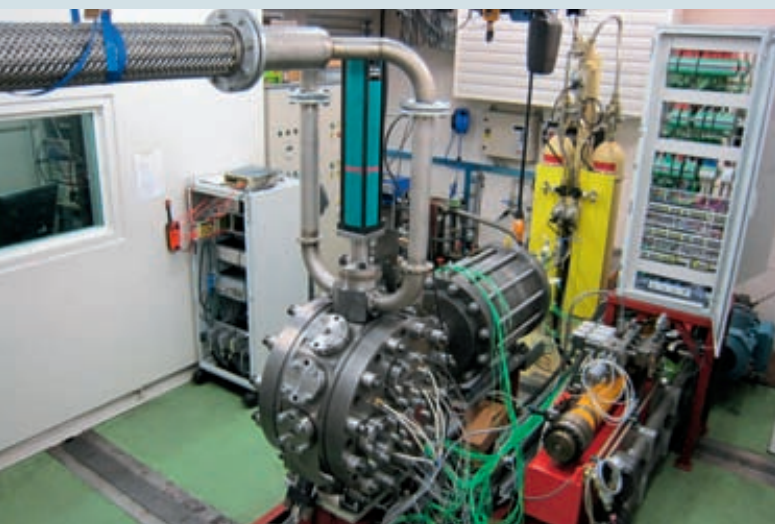
A test stand for combustion systems of large 2-cycle ship diesel motors; EU-Project Hercules.
