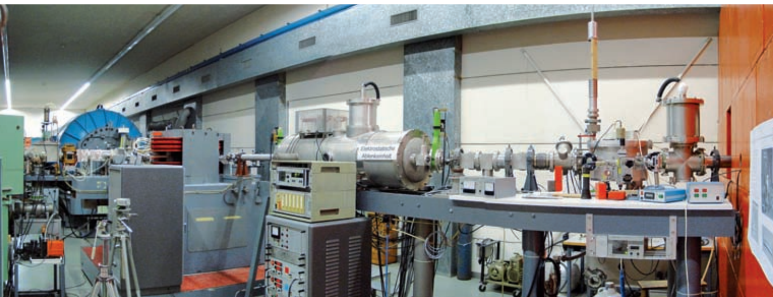
With the TANDEM accelerator of the ETH Zurich deterioration of materials caused by radiation is induced to anticipate the performance of future nuclear plants. After the irradiation of materials, correlations between their material properties and microstructures are investigated at the PSI.
