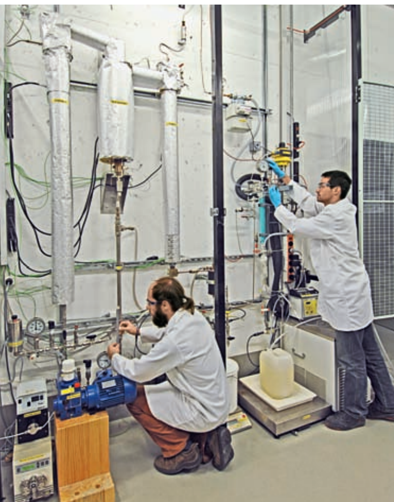
The catalytic hydrothermal gasification of biomass is being investigated at the Paul Scherrer Institute in Villigen. Continuous operation is being tested in a laboratory set-up with capacity of 1 kg/h. Typical operating conditions are 400°C and 30 MPa
